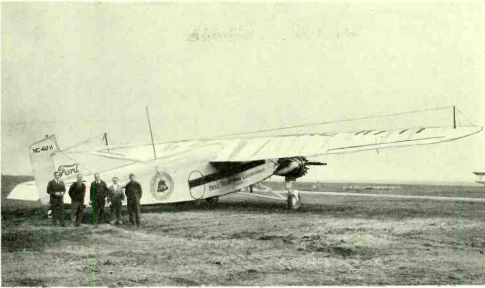
Fig. 3—The Ford tri-motored plane with fixed V and strut antennas. Standing beside it are the Laboratories pilots, Capt. A. R. Brooks and P. D. Lucas, and the ground crew: left to right, R. Zilch, C. T. Garner, and Walter Funda
