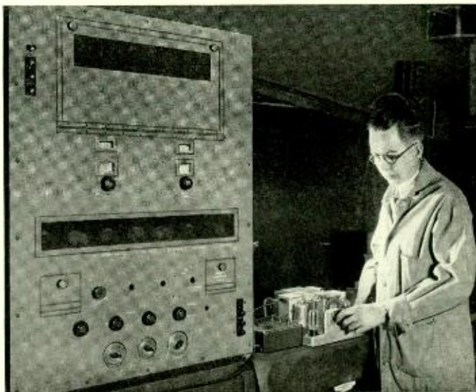
Fig. 3—H. B. Fischer testing a 9-A radio receiver in the shielded room
