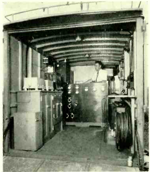
Fig. 2—Within the body is complete radio equipment of the type used in both aircraft and ground terminals
