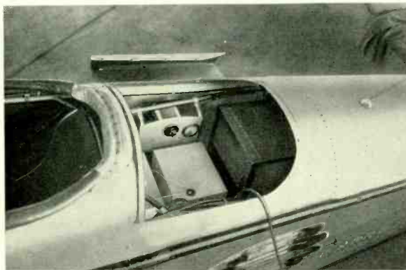
Cock-pit of mail plane of the Western Air Express showing control equipment for Western Electric aircraft radio system
