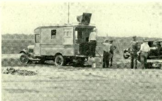
Fig. 3—Truck-mounted portable radio station for aircraft survey work
