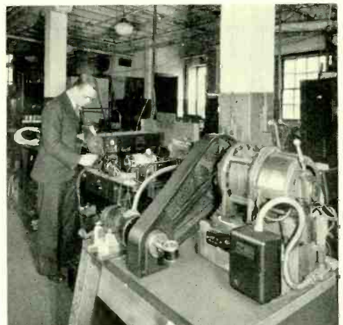
Fig. 2—F. C. Ward conducting a test on an engine-driven generator
