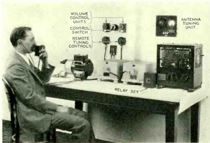
Fig. 1—E. F. Brooke with complete radio-telephone equipment for airplanes
