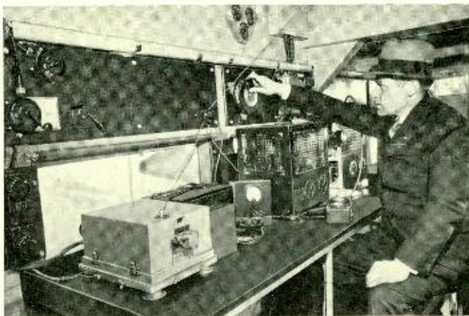
Fig. 6—In the Ford plane is a laboratory bench for experimental apparatus. F. S. Bernhard is shown making an antenna test
