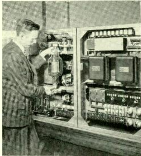
Fig. 9—Rear view of the ground transmitter and power cabinets. A 251-A tube is being inserted by J. B. Bishop
