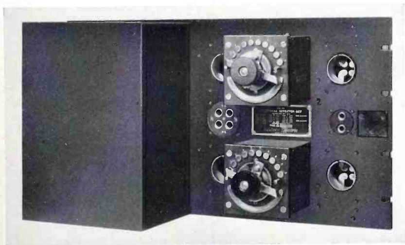
Fig. 8—A single panel of 44-A-1 repeater showing dials for gain adjustment
