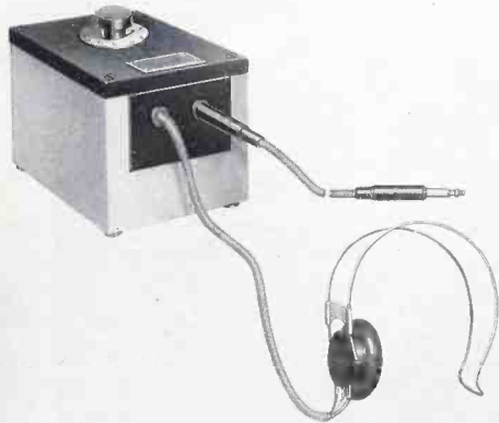
Fig. 3—Adjustments of the continuity bridge are made by a potentiometer in the portable test box. A head receiver serves as the detector
