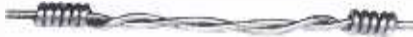
Fig. 1—The Western Union joint is easily made and for many years was standard for open-wire telegraph construction
