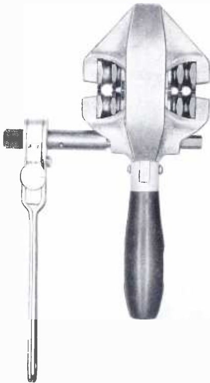
Fig. 4—The rolling tool, equipped to join four sizes of wire, weighs but four pounds and is thus easily handled aloft
