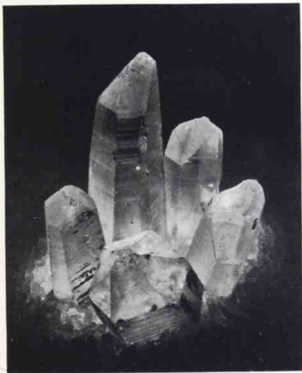
Quartz crystals, from which plates are cut for frequency control, pictured by the Photographic Department against a background of small ("hypo") crystals
