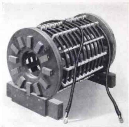
Fig. 6—One of the smaller coils, 20 inches in diameter, 33 inches long, has an inductance of 28 microhenries. It appears in the upper right-hand corner of Fig. 5
