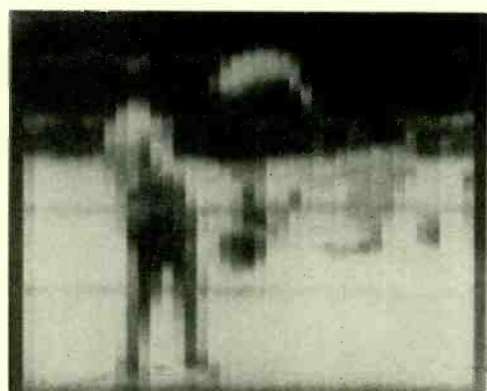
Fig. 3—With two ordinary broadcast channels, 1250 elements could be transmitted. The gain over Fig. 2 is obvious
