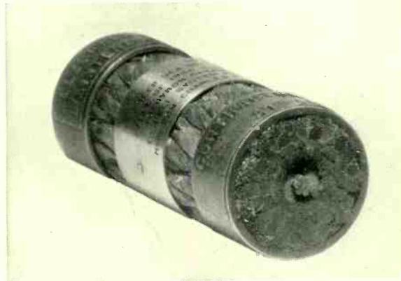
Deep sea section of the first successful Atlantic telegraph cable, laid in 1866. The core consists of a strand of seven copper wires each of No. 18 B.W.G., coated with four layers of gutta-percha alternating with four of Chatterton's compound. Next is a cushion of tanned jute and over this there are wound spirally ten homogeneous galvanized iron wires No. 13 B.W.G. Each wire is separately covered with five strands of Manila yarn
