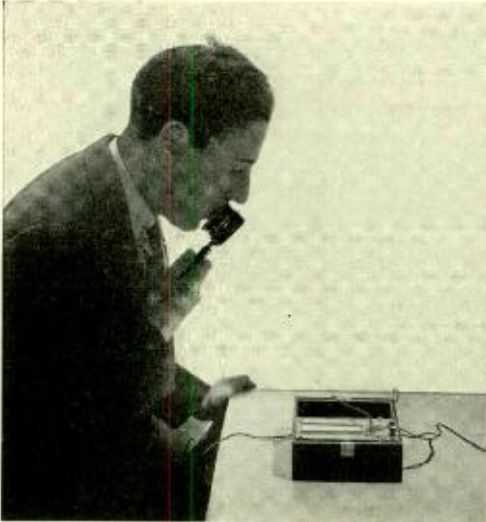
In the Acoustical Laboratories speech waves are analyzed by the tuned-reed harmonic analyzer which A. Grieco is using
