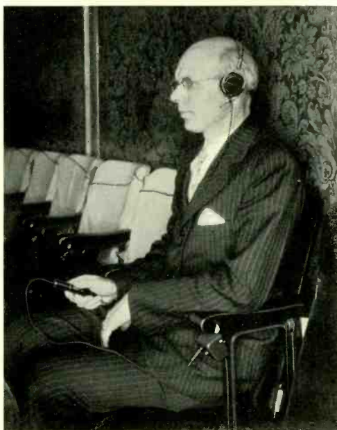
Fig. 3—The cord is plugged into the jack under the arm of the seat and the intensity of sound is controlled by the potentiometer in the hand of the listener
