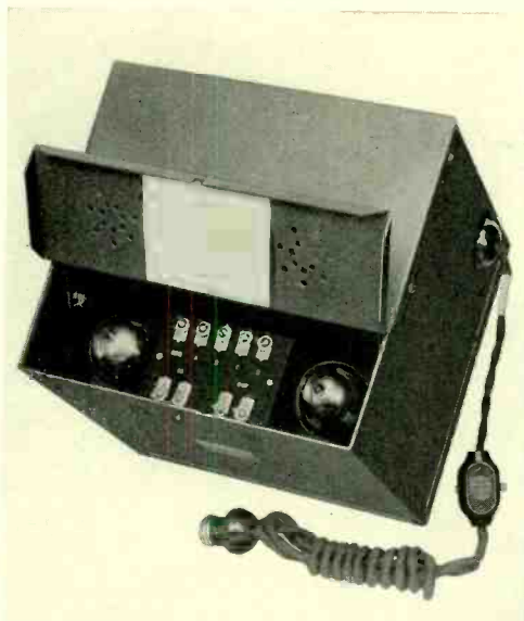
Fig. 2—The No. 51-A amplifier used in the theatre deaf system. It supplies thirty individual sets
