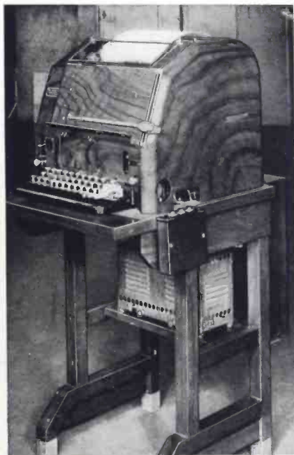
Fig. 3—The teletypewriter both sends and receives, producing records of all messages at both ends of the call. The only special controls which must be added to the standard teletypewriter to equip it for the new service are three push-button keys for "call," "answer," and "recall," mounted on the right hand side. The box behind contains the ringer, and relays associated with the push-button keys
