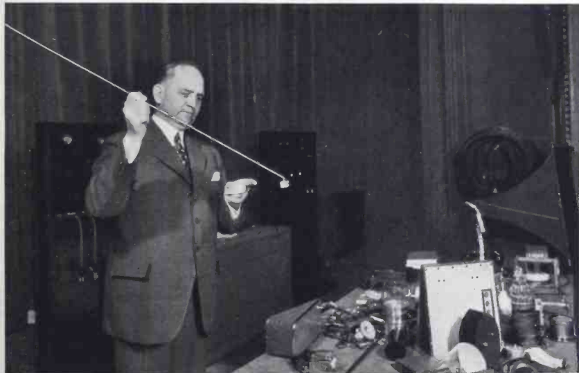
How a permalloy rod responds to the earth's magnetic field is a demonstration often made by Mr. Grace. Proper orientation of the rod determines whether it will pick up a thin sheet of permalloy or let it fall. Mr. Grace has recently addressed enthusiastic audiences in Chicago, Urbana and Springfield, Illinois
