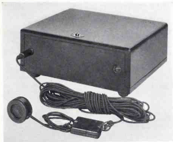
Fig. 3—Associated with the lapel microphone, an input circuit attenuates the lower frequencies which the microphone picks up from the speaker's chest, and prevents clicks when the microphone is cut in or out of circuit
