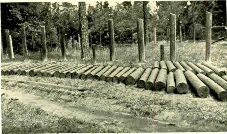
Fig. 4—These treated specimens are ready to be set in the ground for test at the Gulfport plot
