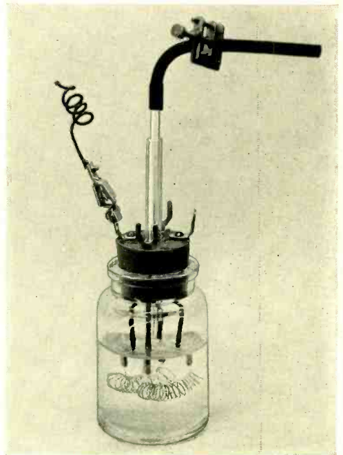
Fig. 5—The corrosiveness of a liquid toward a metal can be determined by measuring the change in resistance of wires when immersed in the liquid
