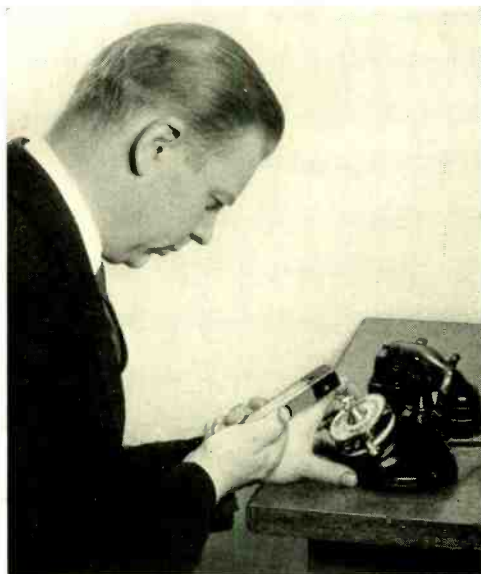
Fig. 3—S. J. Stockfleth demonstrates the use of the stroboscope for checking the speed of a subscriber's dial
