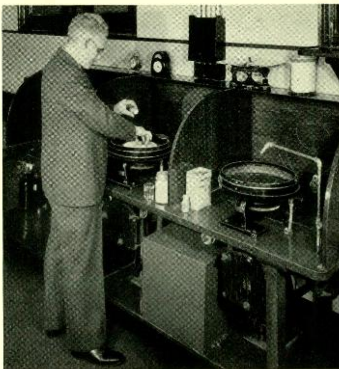
Fig. 2—The final polishing operation is carried out on horizontal laps covered with broadcloth which is stretched tight and wet with a thin paste of alundum powder and water. R. M. Sample is demonstrating the method
