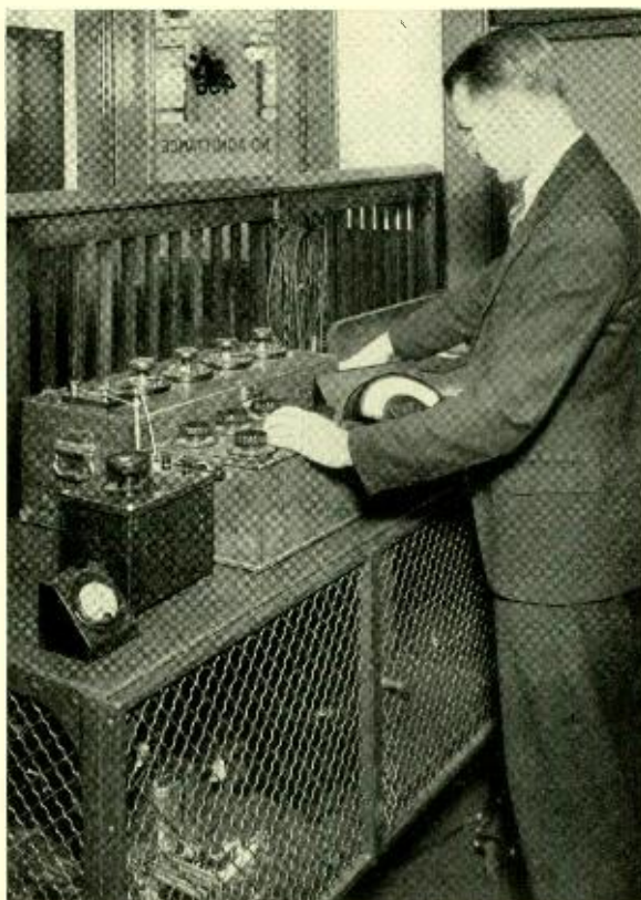
Fig. 1—Making a measurement of inductance with the new measuring circuit
