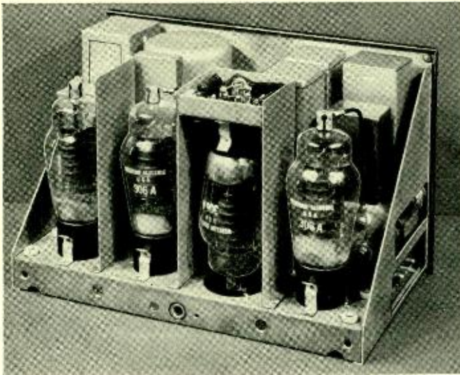
Fig. 1—Rear view of the chassis of the 18A Radio Transmitter. The harmonic generator tube is inverted to shorten the leads
