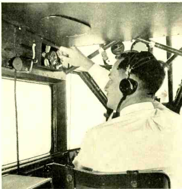
Fig. 3—The 27A control unit as installed in the Fairchild plane of the Laboratories
