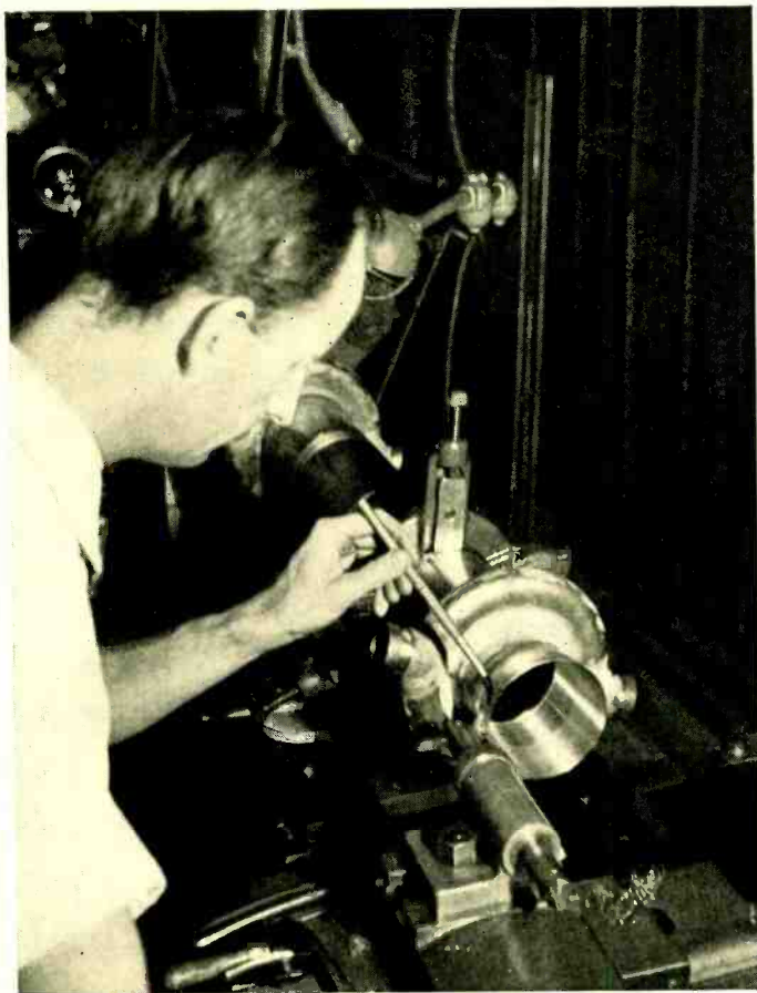
Machining the edge of a copper anode where it is to be sealed to glass for an experimental 250-kilowatt triode
