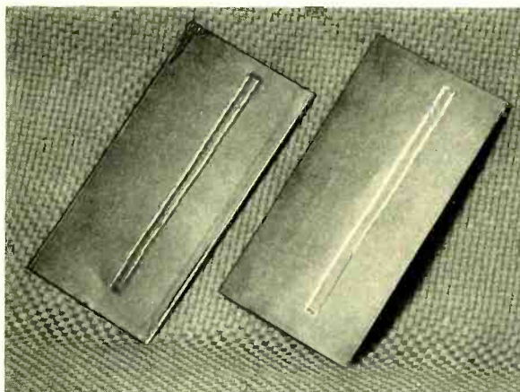
Fig. 3—The left panel was struck a series of blows of constant intensity. Breakdown under blows of increasing severity is shown by the change of color in the path of the hammer on the right panel
