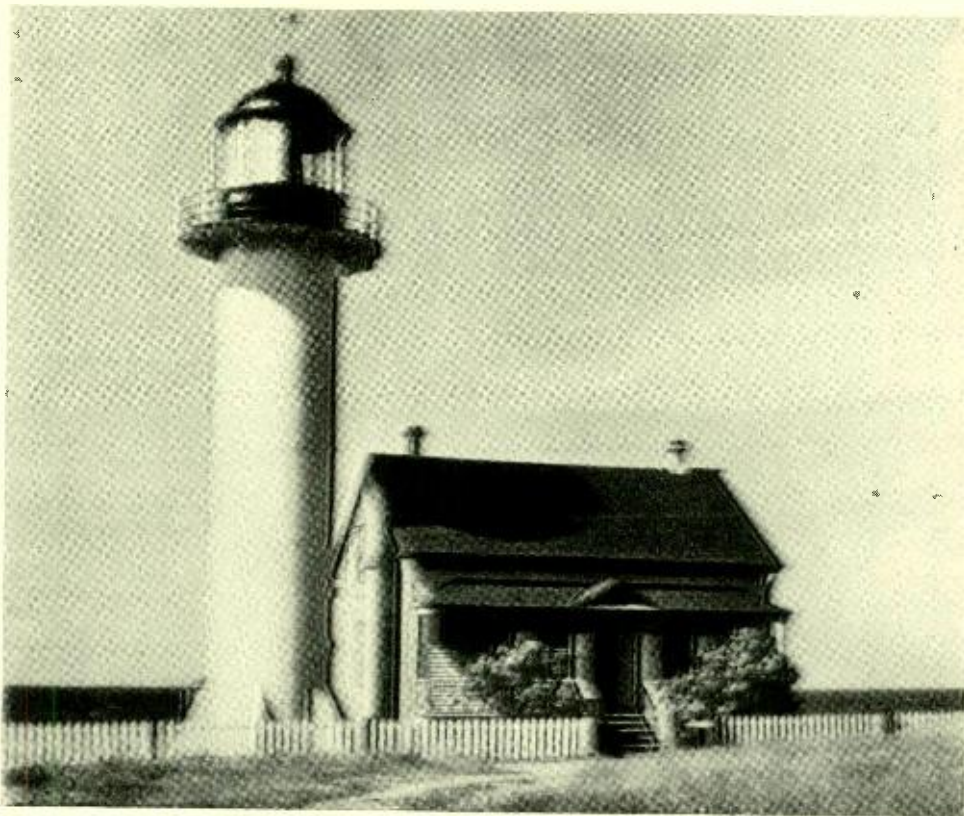
Fig. 1—The result of transmitting the photograph shown at the head of this article over a toll line not specially arranged for telephotograph transmission
