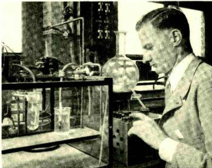
Fig. 4—The amount of soluble salt in paper is found from the electrical conductivity of a water extract of the sample. W. G. Guldner is making the test
