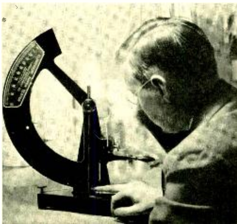
Fig. 3—The toughness of paper is evaluated by measuring the difference in height reached by a pendulum when swinging freely and when it tears a strip of paper
