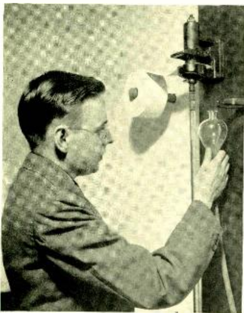
Fig. 2—The density of paper is determined by measuring its porosity, done by finding the rate at which air diffuses through it
