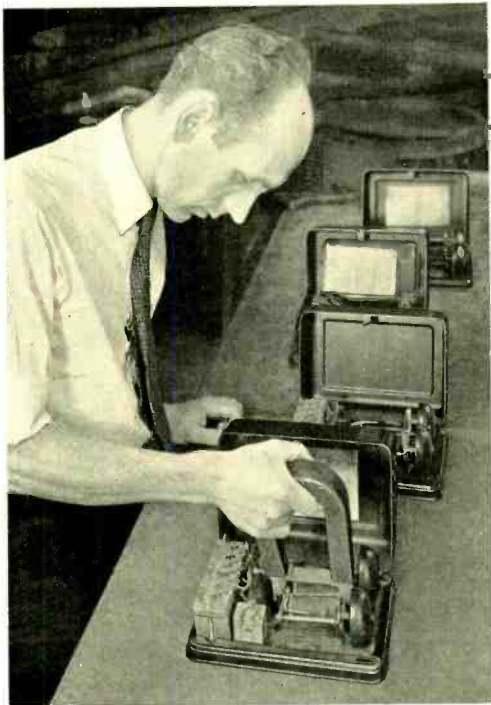
Fig. 1—The remagnetizer can be used on ringers assembled in the subscriber sets housed in metal and phenol plastic boxes
