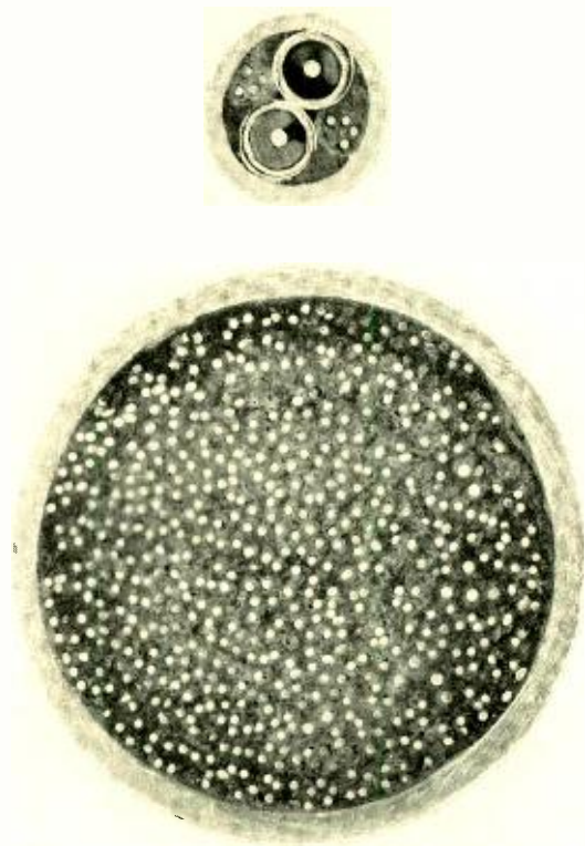
Fig. 1—The coaxial cable occupies but one-ninth of the space required for a full size toll cable
