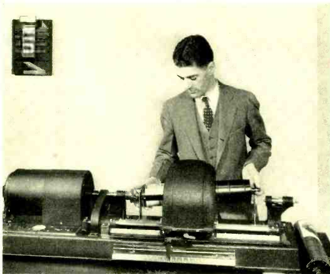
Fig. 1—The telephotograph transmitter showing the cylinder being removed after the transmission of a picture
