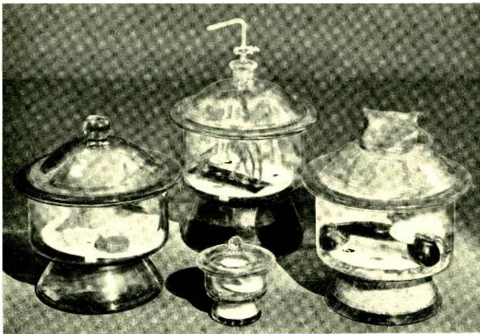
Fig. 1—Air conditioning tests can be made in desiccator jars. The humidity of the air is controlled by the solution in the base of the jar
