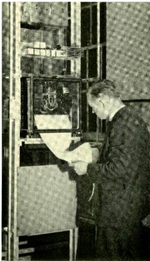
Fig. 6—M. M. Bower with the recorder that is used for measuring the resistance of the pilot wire during the trial period
