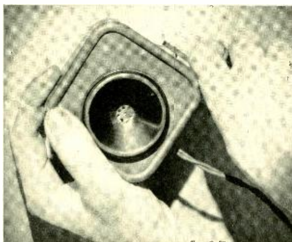
Fig. 4—The combined transmitter and receiver is three inches square and weighs less than two pounds
