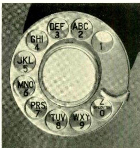
Fig. 4—This dial for colored handsets has stainless steel finger wheel and finger stop
