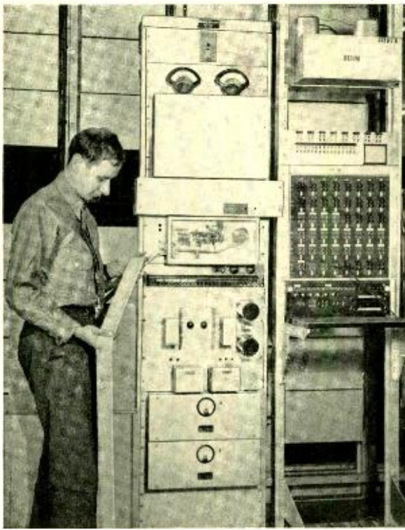
Fig. 5—J. P. Kinzer at the automatic transmission-measuring set, which measures net loss of complete circuit from 12 to 60 kilocycles in fifteen seconds. The sealed terminal bay is located at the right
