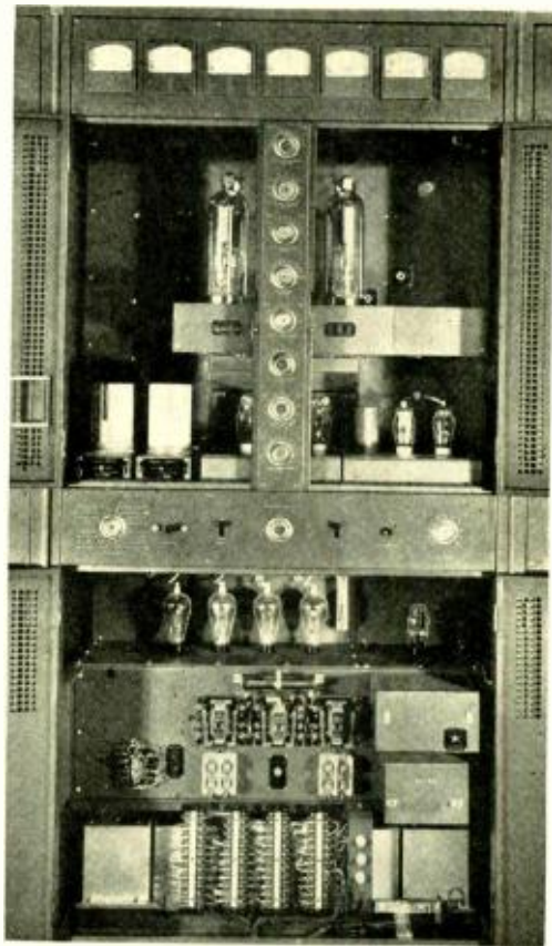
Fig. 2—The oscillator-modulator unit with front doors open. The two crystals are at the left in the upper compartment
