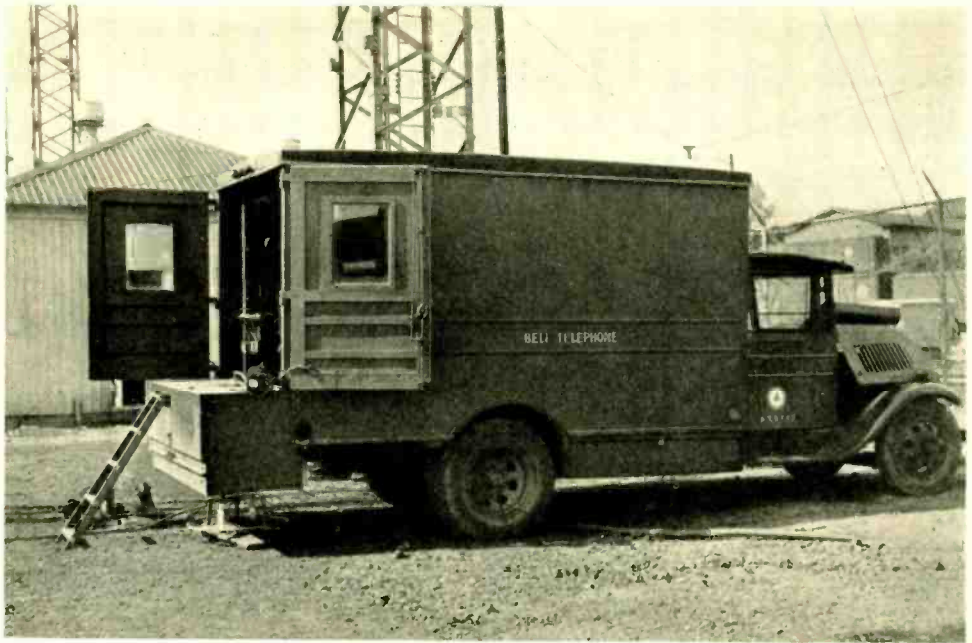
Fig. 2—This truck contains an electric power plant for testing
