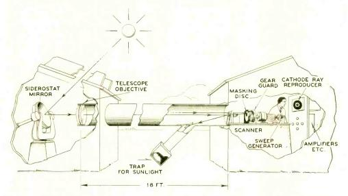
Fig. 1—This diagram shows the application of the Coronaviser to a horizontal telescore February 1940 163
