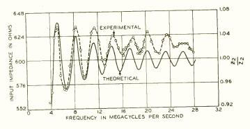
Fig. 3—Input impedance of an exponential line with series inductance to compensate for stray capacity at the terminals. The difference between the theoretical and experimental curves is due to deviation at high frequencies of the comparison resistance from its direct current values
