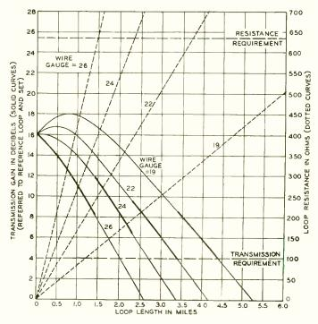
Fig. 1—Transmission loss in subscriber loops for various gauges and lengths of loop
