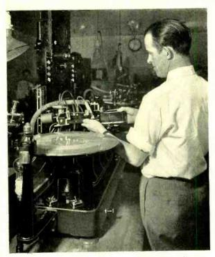
chanical motion to cut a record on a disc or cylinder for later reproduction. Such recordings are used extensively, both for sound pictures and for the electrical transcriptions used widely in broadcast programs.
