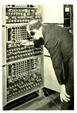
Fig. 4—A terminating sender under test in the systems laboratory
