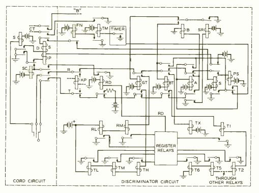
Fig. 1—Simplified schematic of the testing circuits of the discriminator February 1940
