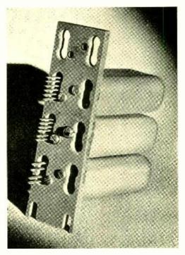
are provided for busy test. In the illustration the 102B induction coil is shown at the top. The middle coil is the 161A monitoring and busy test coil; and below a retardation coil.
