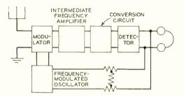
Fig. 4—Simplified block schematic of the Laboratories feedback receiver for frequencymodulated waves
