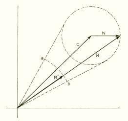
Fig. 3—Noise can be represented by a vector x added to the carrier vector, which produces both phase and amplitude changes in the resultant vector
