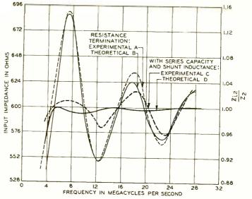
Fig. 4—Input impedance of a 600 to 300-ohm exponential line fifteen meters long with a resistance termination; also with a series capacity at the high impedance end and an inductance shunted across the resistance at the low impedance end
