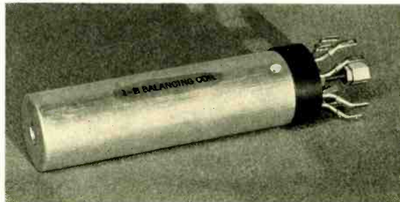
Fig. 4—Assembled 1B balancing coil showing adjusting nut and rod at the right
