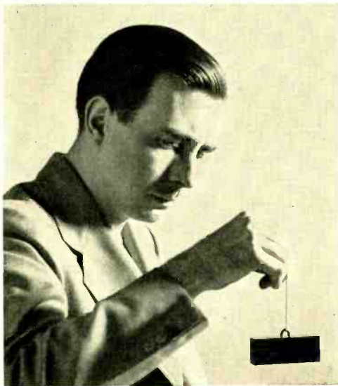
E. A. Nesbitt holds up two iron bars by the magnetism stored in the little semicircular magnet made from "Vicalloy"
