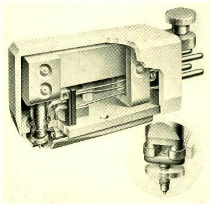
*Fig. 2—The two pick-up coils are wound on a duralumin cup. A flat triangular spring between these coils supports them and the stylus. This spring flexes readily up or down but not sideways because of the wide cross section of the coils, thus restricting all motions except the lift required for vertical reproduction and the rotation of lateral reproduction*
