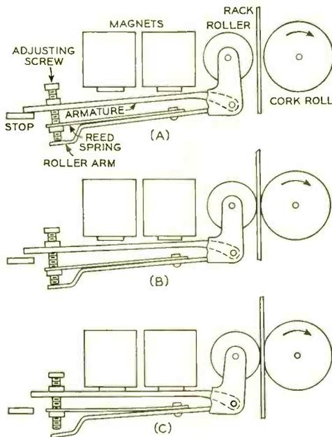
Fig. 1—Diagrammatic representation of the original clutch from the open position, above, to the fully operated position, below
