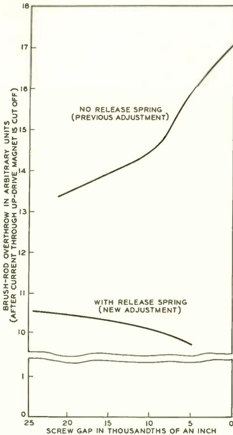
Fig. 3—Brush overtravel for various screw-gap openings with and without the spring
