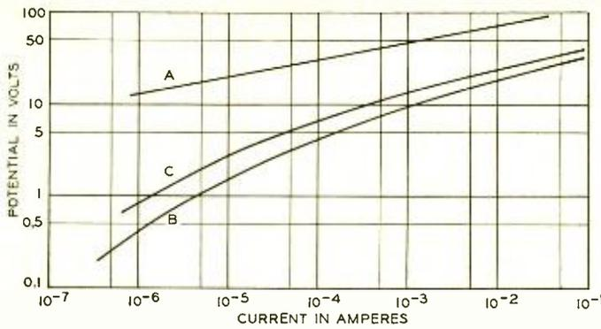
Fig. 2—Characteristic curves for varistors 0.045 inch thick and 1.3 square inches area. Sample A passed through the furnace at 5 minutes per inch; sample B at 15 and sample C at 12 minutes per inch
