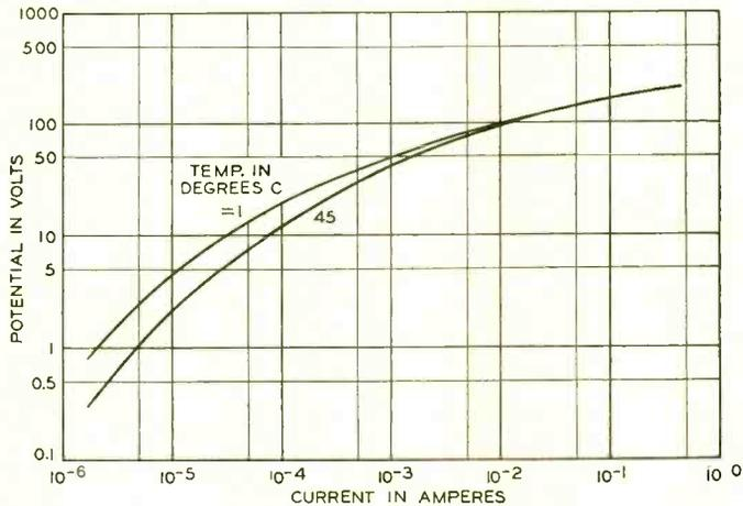
Fig. 7—For the same voltage, current approximately doubles with increase of temperature from 1 degree Centigrade to 45 degrees Centigrade
