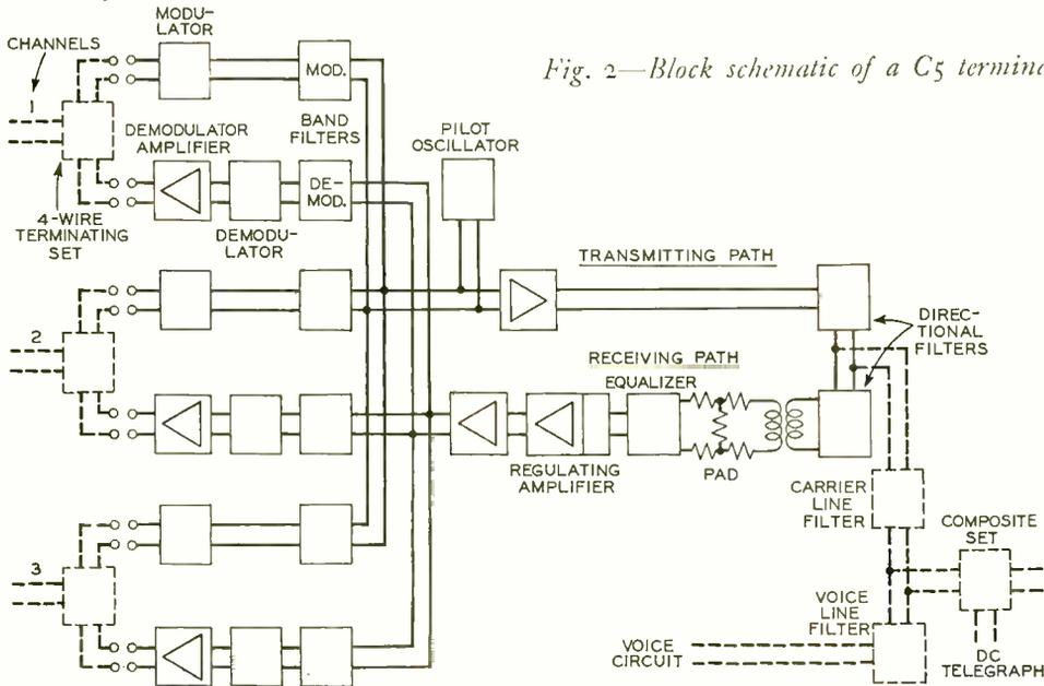
Fig. 2—Block schematic of a C<sub>5</sub> terminal
