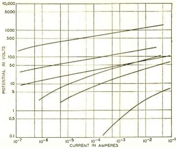
Fig. 5—An indication of the variety of characteristics which can be obtained in silicon carbide varistors
