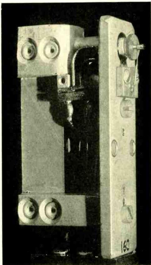
*Fig. 1—The 9A reproducer is very small. Its diamond stylus is at the base of a T lever with minute coils on each arm*
