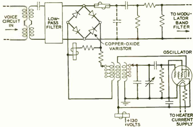
Fig. 3—Simplified schematic of the modulator circuit
