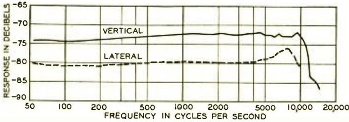
Fig. 3—The response of the 9A reproducer is essentially flat—up to nearly 10,000 cycles per second. It is made more sensitive for vertical reproduction to compensate for the lower level at which vertical-cut records are usually recorded
