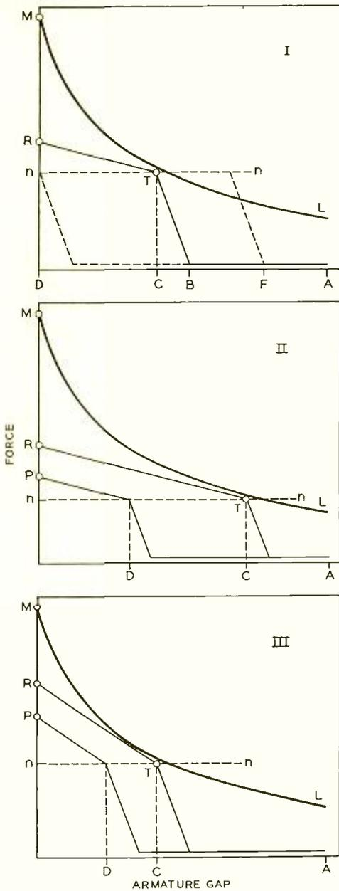
Fig. 2—Force-displacement diagram for the original clutch for various conditions
