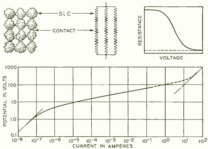
Fig. 1—Electrical characteristics of granular silicon carbide
