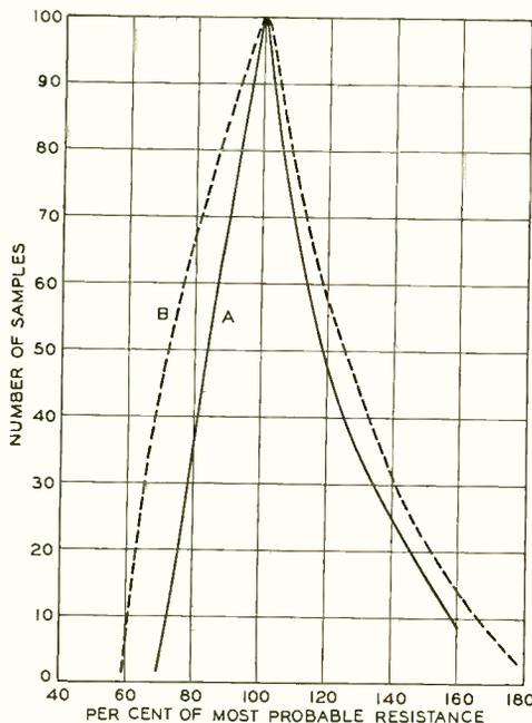
Fig. 6—Characteristic frequency distribution curves: A, when measured at high voltage; B, at low voltage
