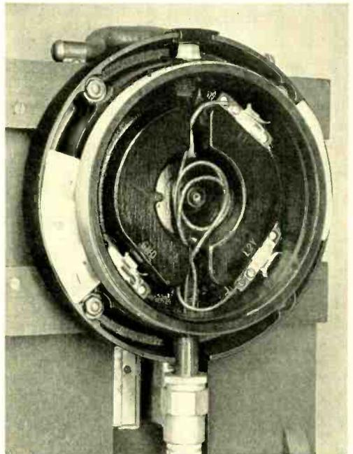
*Fig. 1—The base of the new set provides termination for the wires and is designed to support the housing and to mount on a wall, either directly or by use of a backboard*
