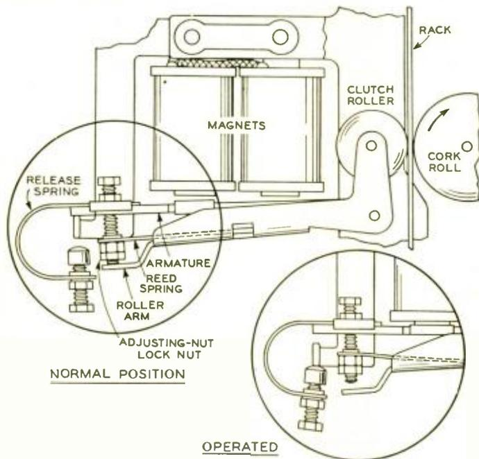
Fig. 2—A clutch equipped with release spring to provide a releasing force regardless of the screw-gap opening
