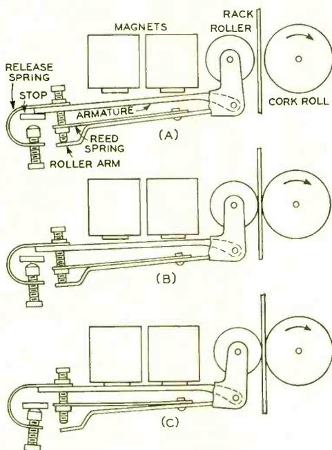
Fig. 3—Diagrammatic representation of the clutch with release spring—open position, above, and fully operated position, below
