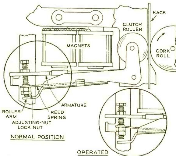
Fig. 1—Arrangement of clutch showing reed spring and adjusting screw
