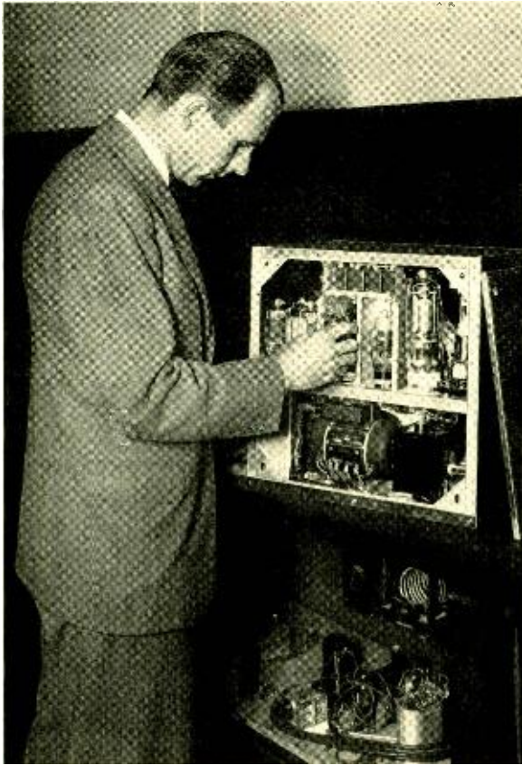
Fig. 4—A. K. Bohren inserts a tube in the new ten-frequency transmitter during an inspection of one of the early samples at the Laboratories
