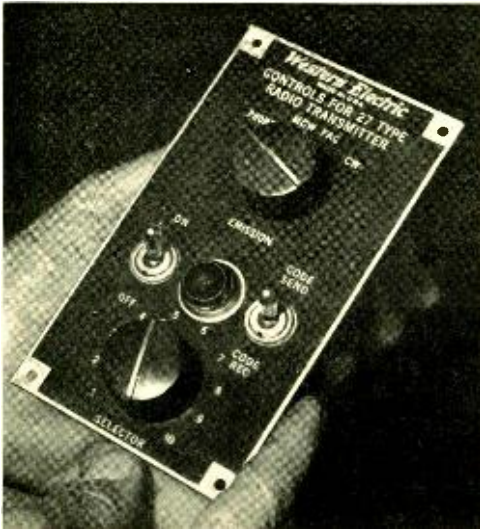
Fig. 2—Remote control unit for the 27-type radio transmitter
