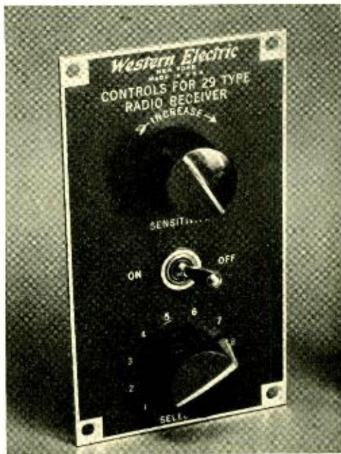
Fig. 3—Remote control unit for the 29A ten-frequency receiver
