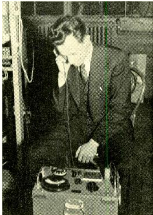
R. D. Fracassi making noise measurements on cable carrier program equipment
