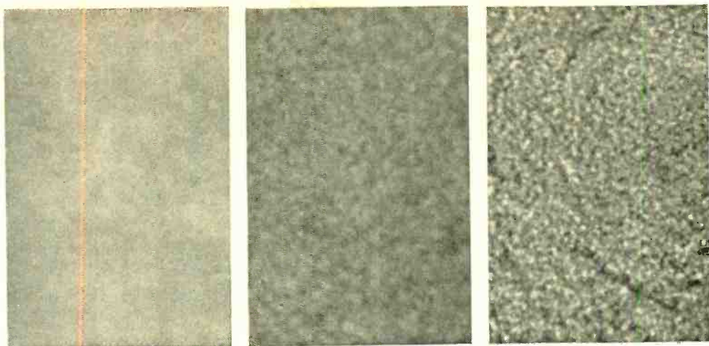
Fig. 1—Photograph of rubber sheets with 3 per cent sulfur: cured immediately after mixing, left; cured after 1 day storage, center; and cured after 11 days storage, right
