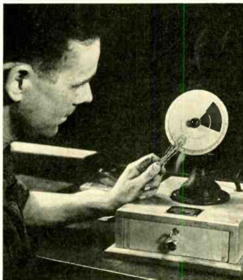
Fig. 3—Color test disks and drive motor as used at the Kearny plant of the Western Electric Company
