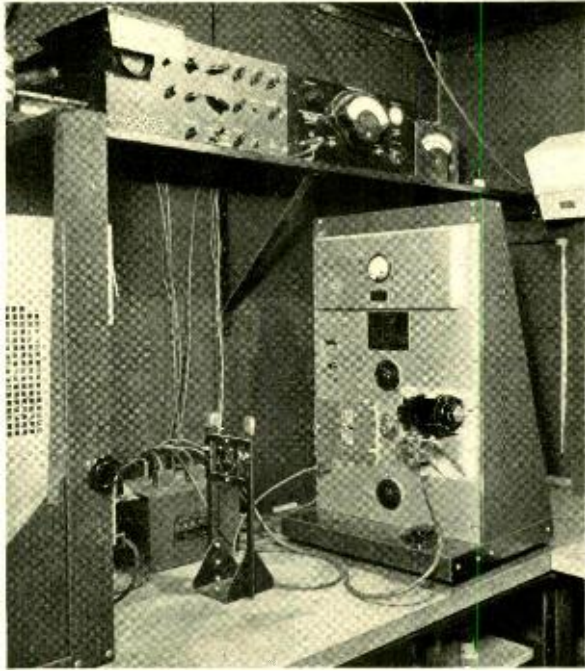
Fig. 4—A 17B oscillator ready for calibration in the calibration dark-room at the Kearny plant of the Western Electric Company
