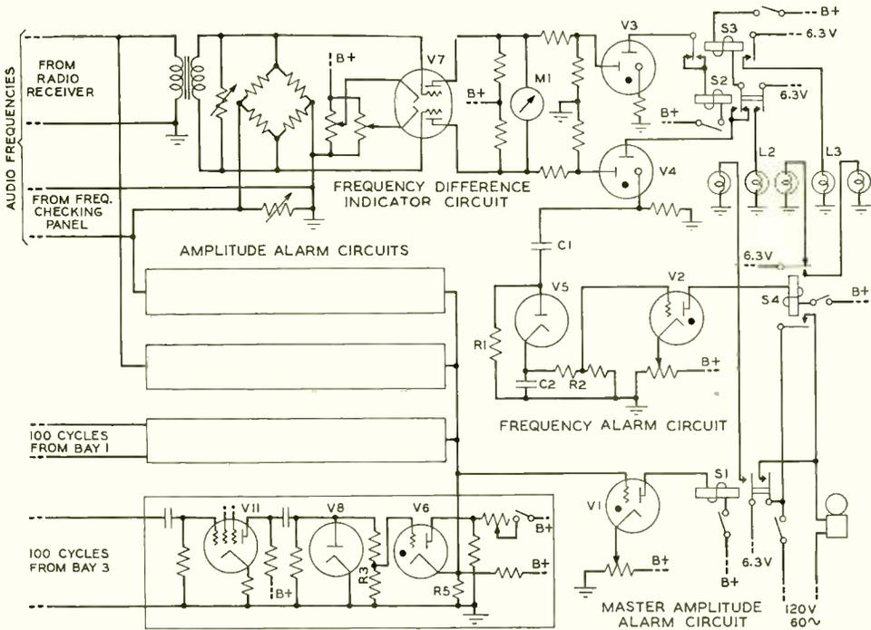
Fig. 2—Alarm and comparison circuit
