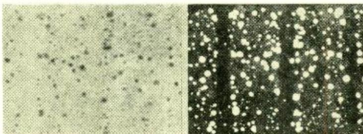
*Fig. 1—Photographs of condenser paper broken down by acid liberated from the impregnant: (left) illuminated by ordinary light, (right) with ultraviolet light*
