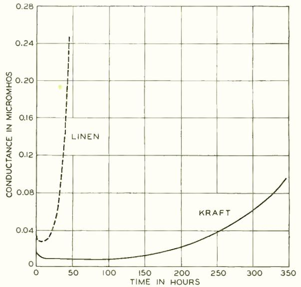
Fig. 4—Leakage current in condensers under accelerated life test remains small much longer with Kraft paper than with linen paper insulation
