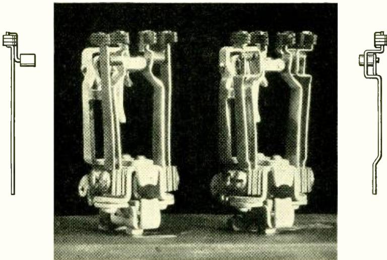
*Fig. 1—Selector brushes with flexibly mounted shoes (right) cause less circuit noise than those with straight springs (left). The outside springs of the older type are straight while those of the new type have a U bend near the shoes*
