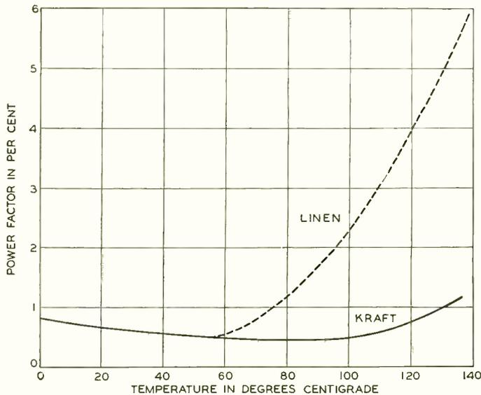
Fig. 3—Energy loss at high temperatures is less in condensers that are made with Kraft paper than it is in those in which linen paper insulation is used
