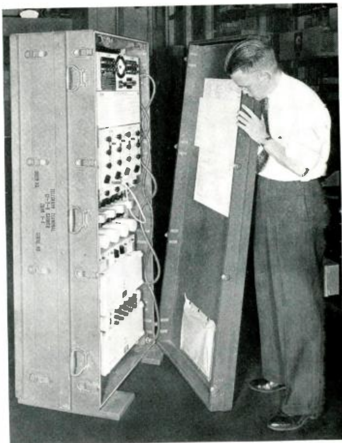
Fig. 1—Covers may be placed on the terminal in a very few moments without the aid of special tools
