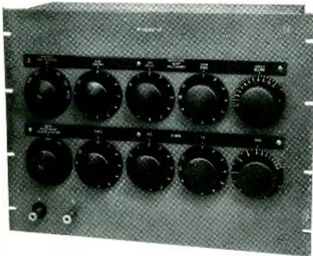
Fig. 1—Maxwell type bridge used for measuring the resistance and inductance
