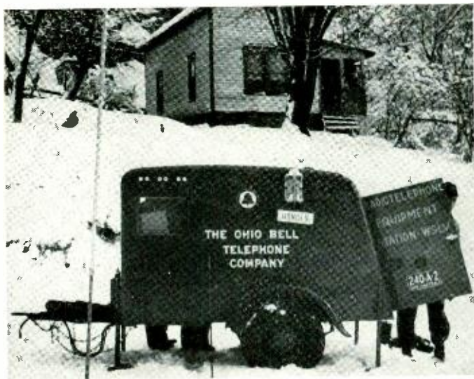
Useful in bridging many a storm break are the hundred portable radio stations owned by Bell System companies. Pictured above is one end of a 27-mile radio link set up near McConnellsville, Ohio, to bring the town of Marietta back into the telephone network. A development of the Laboratories, this equipment has 50 watts transmitter power
