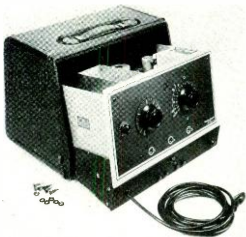
Fig. 2—The face of the 6BP audiometer is tilted up to facilitate operation
