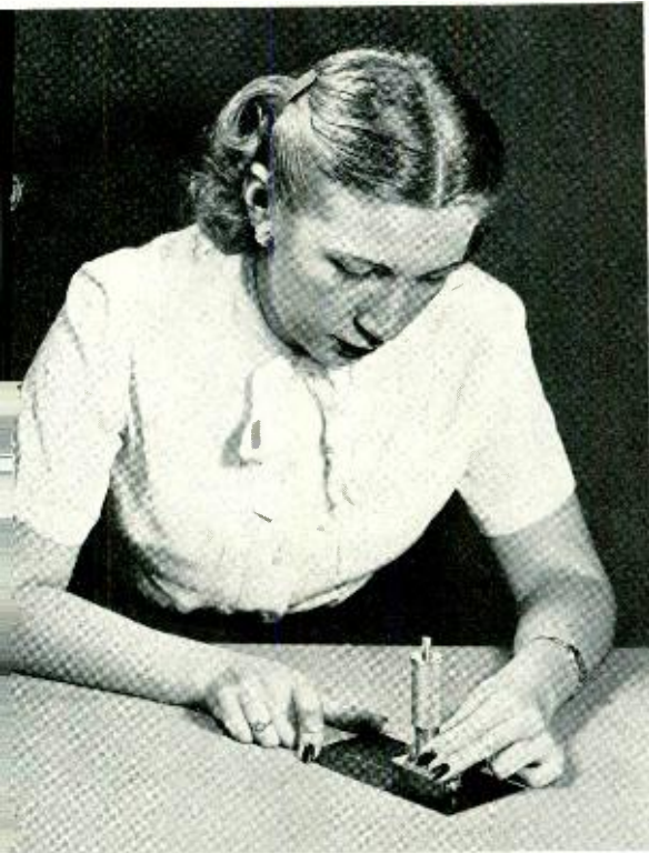
Testing to determine optimum adhesional quality of a finish coating
