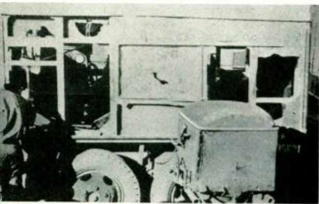
The most severe test of all couldn't stop this M-9. During the defense of Antwerp, a V-1 buzz-bomb exploded thirty feet away. Heat from the blast fused parts of the optical tracker. The M-9 computer inside the trailer continued to function perfectly without repair
