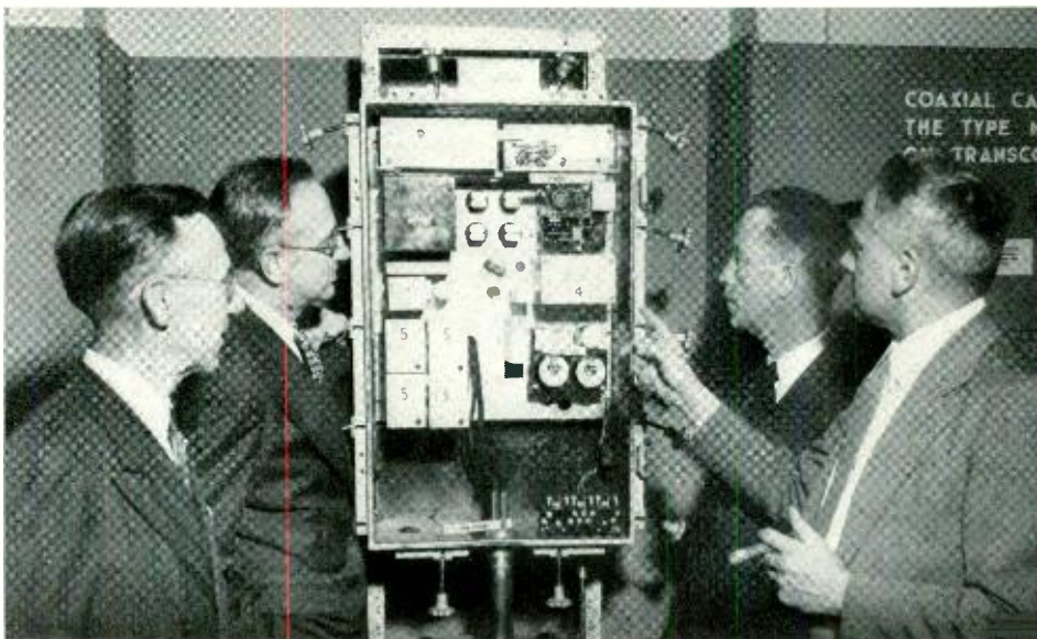
At the Television Broadcasters' Convention, J. F. Wentz, Ralph Bown, A. B. Clark and J. R. Wilson inspect a coaxial cable repeater
