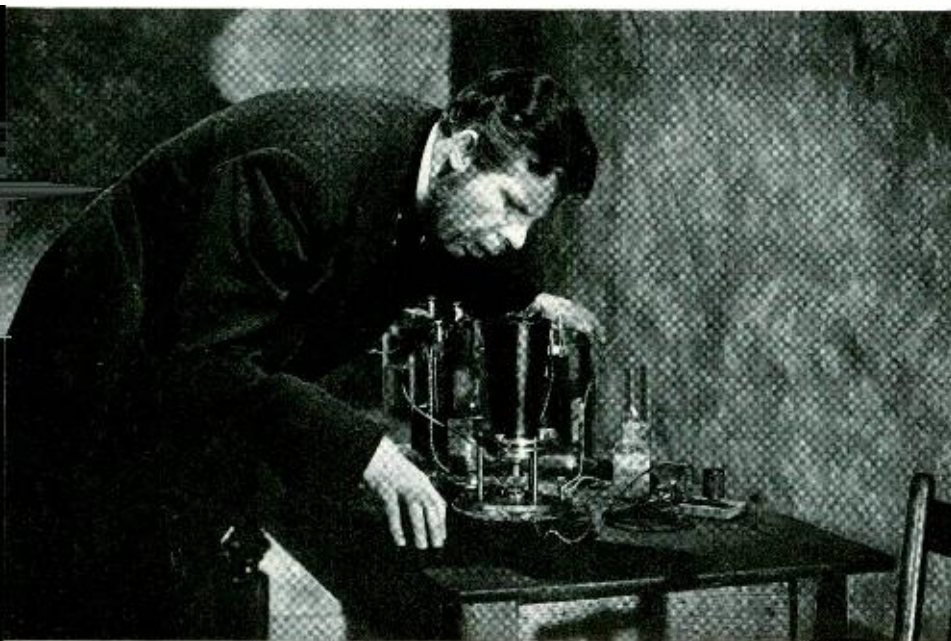
Needing more energy to transmit speech, Mr. Bell made his "liquid transmitter," whose diaphragm had a platinum wire dipping into a small cup of acid
