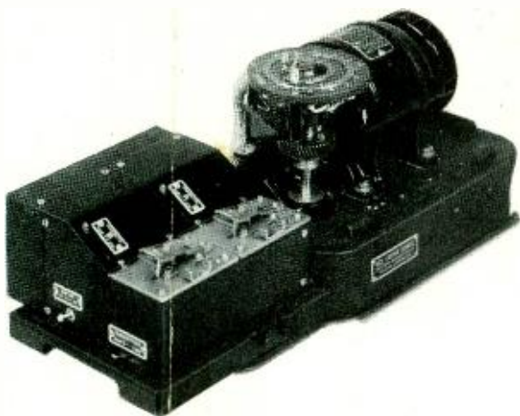
Transmitter-distributor for the two-channel system developed by the Teletype Corporation
