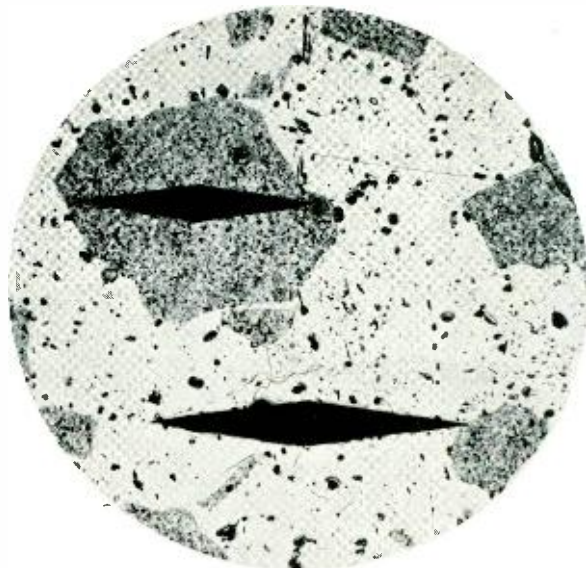
Fig. 5—Knoop indentations for determining hardness of structural areas in a lead-antimony alloy. The magnification in this case was 250
