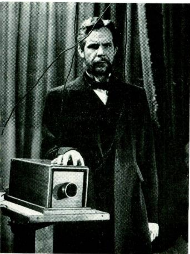
At a lecture demonstration that was held in New York City, music and speech transmitted from New Brunswick were heard by the audience. Pictured is the identical "box telephone," now in our Bell System Historical Museum at West Street
