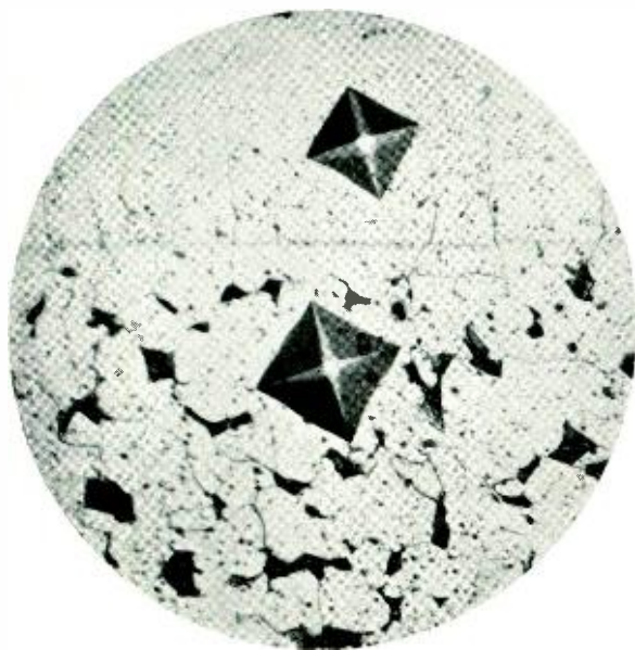
Fig. 4—Vickers indentations in a diffusion layer of an iron-aluminum alloy (top) and in the low carbon steel base material (bottom). Magnification 500
