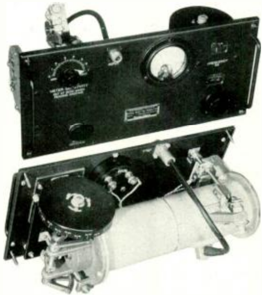
Front view of echo box panel, above, and rear view of panel showing echo box, below
