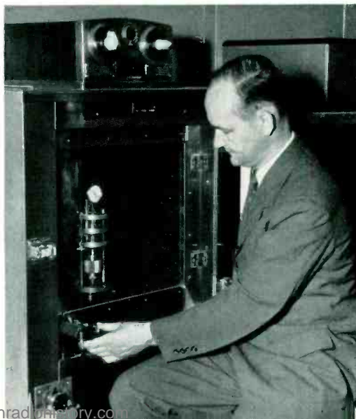
Fig. 3—To insure that the material was hard enough to withstand temperatures of 120 degrees F without deforming excessively, the depth of penetration into a sample of rubber thermoplastic in one minute of a weighted rod was determined. C. V. Lundberg tests a sample in the thermostatically controlled oven
