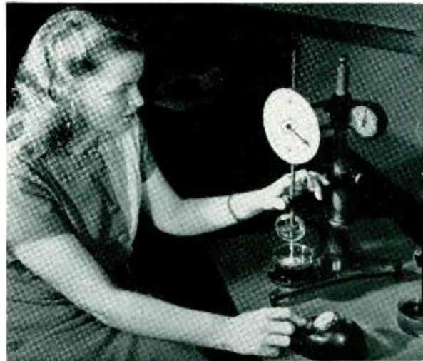
Fig. 5—Viscosity of the adhesive was measured by the rate of penetration of a flat bottomed plunger into a sample of the thick fluid. Doris Smith conducts the test
