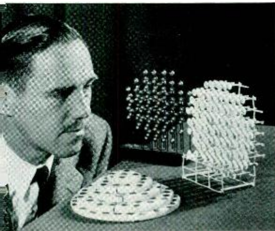
Fig. 1--The author examining lenses of various types: front, a foil disk array supported by dielectric foam; right, conducting disks mounted on rods; and rear, a sphere array
