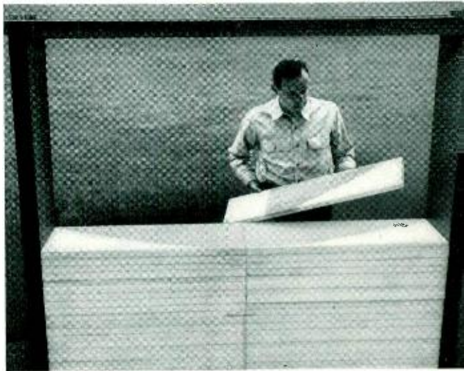
Fig. 5—A six-foot strip lens half assembled
