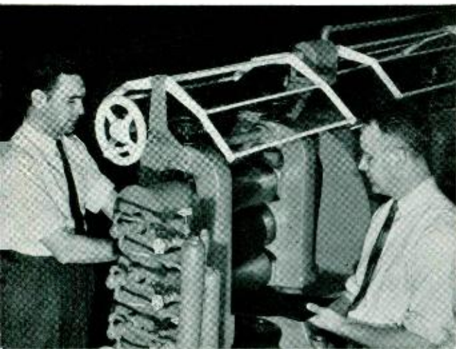
Fig. 1—Processability of the rubber thermoplastic material was determined by calendaring samples into thin sheets. B. Stiratelli (left) and C. M. Hill (right)
