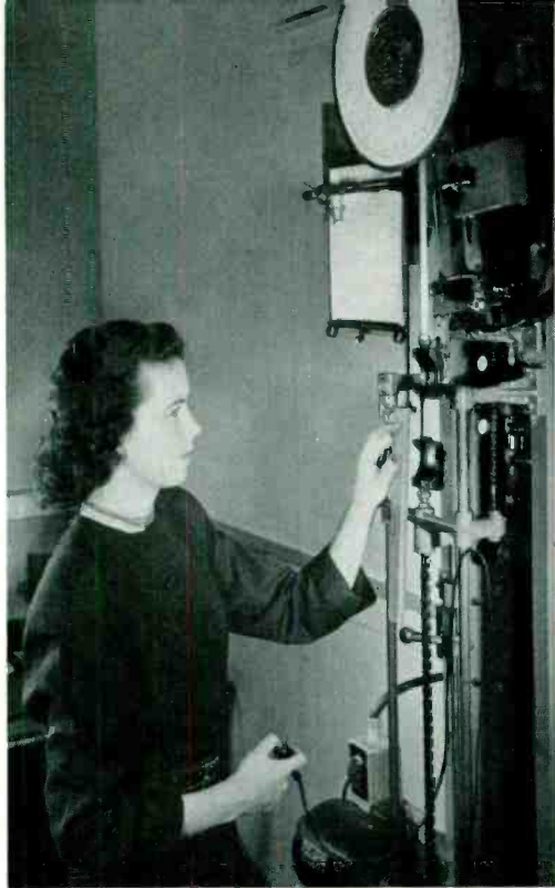
Fig. 2—Tensile strength and elongation were measured by stretching samples on a pendulum-type testing machine. Jean Sanderson is making the test
