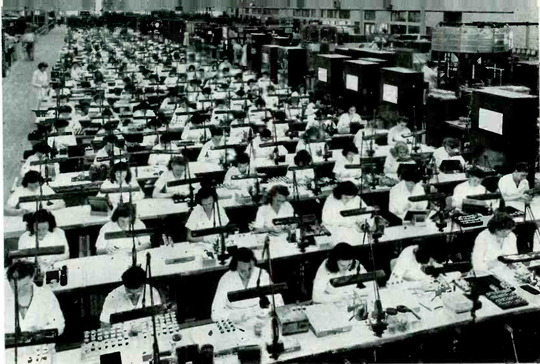
On the main floor, these Western Electric girls are assembling miniature and repeater tubes
