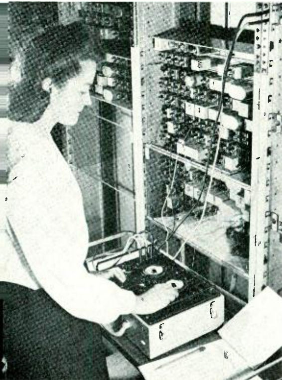
Fig. 1—Cold-cathode-tube test set in use in the systems laboratory
