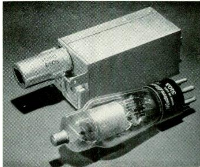
Fig. 1—The V3 repeater with one of the tubes from the V1 repeater in front of it for comparison
