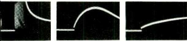
Fig. 4—Oscillograms of voltage at contacts during opening. At left, an unprotected contact; middle, a contact protected with a 184-type network; and at right, a contact protected with the 181-type network. Duration of each trace, 1.5 milliseconds
