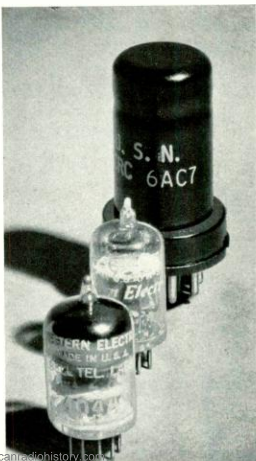
Fig. 1—The Western Electric 404A vacuum tube, at the left, as it appears relative to the 6AK5 and the 6AC7
