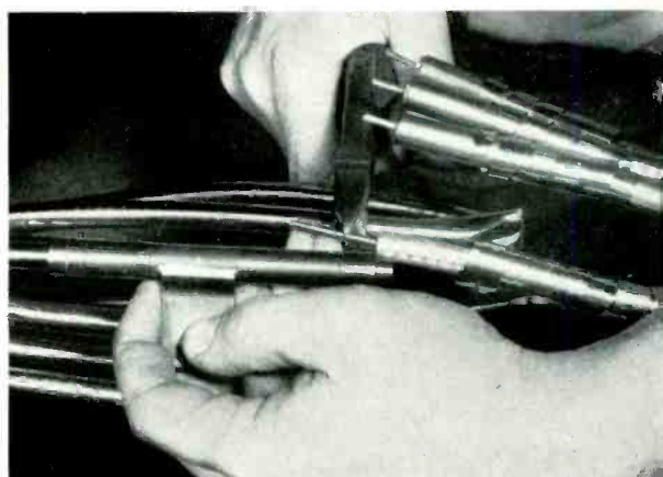
Fig. 5—The inner conductor is cut to project ½ inch from the outer one
