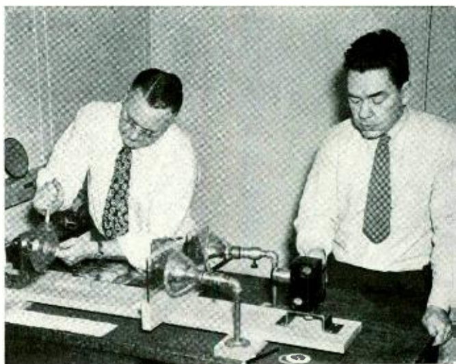
N. R. Pape and I. L. Hopkins making biaxial stress and strain tests on polyethylene in the chemical laboratories at Murray Hill
