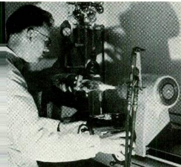
Fig. 1—Shaping a bulb on a glass lathe in the glass-working room
