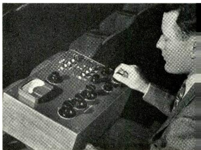
Fig. 4—Important controls of backstage panels are duplicated in a Listening Room console. J. Z. Menard is the operator.
