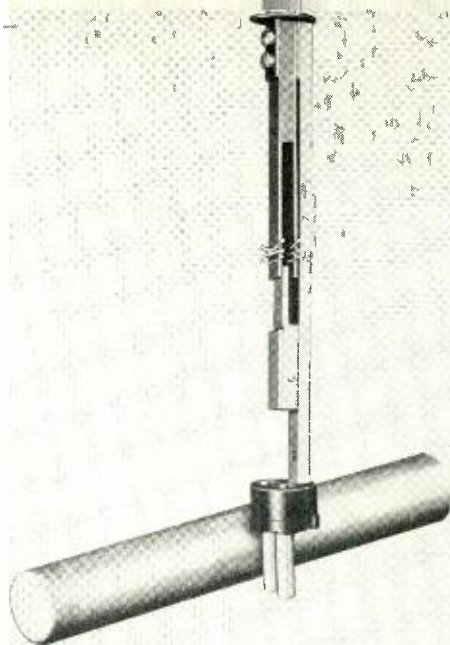
Fig. 6—The vibrating reed unit as used in a filter.
