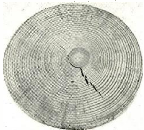
Fig. 2—Photograph of cross-sectional face of untreated southern pine showing spring and summer growth bands.
