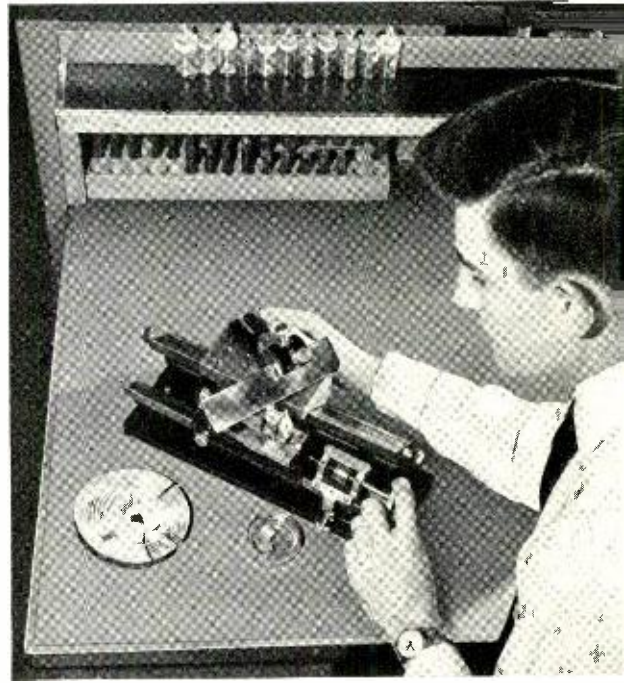
Slices of wood are cut with a microtome for Geiger counter tests.
