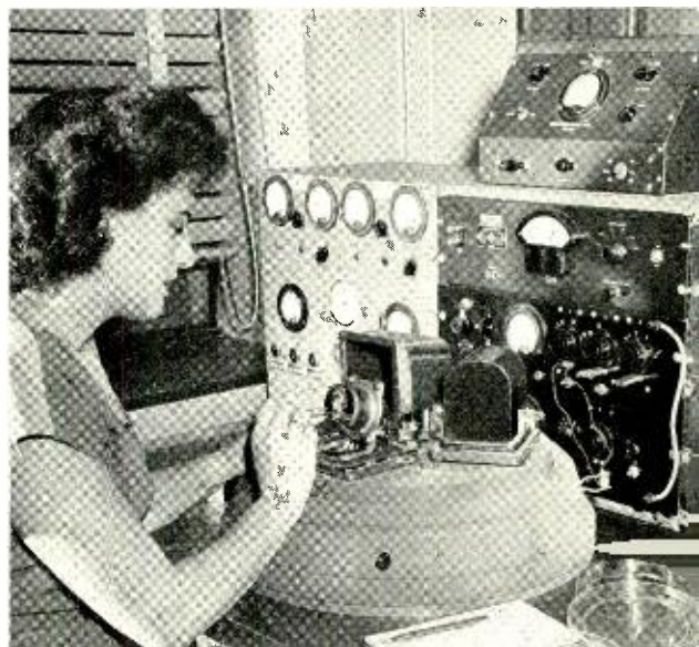
Fig. 2—One of the crystal plating units in the Laboratories.
