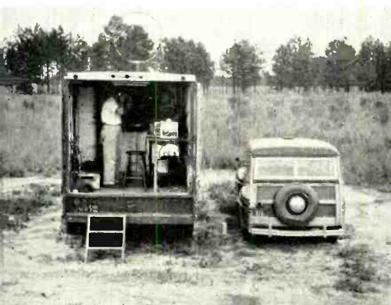
The test truck, with its loop antenna on the roof for direct measurements of static, was stationed 5 miles east of Madison.
