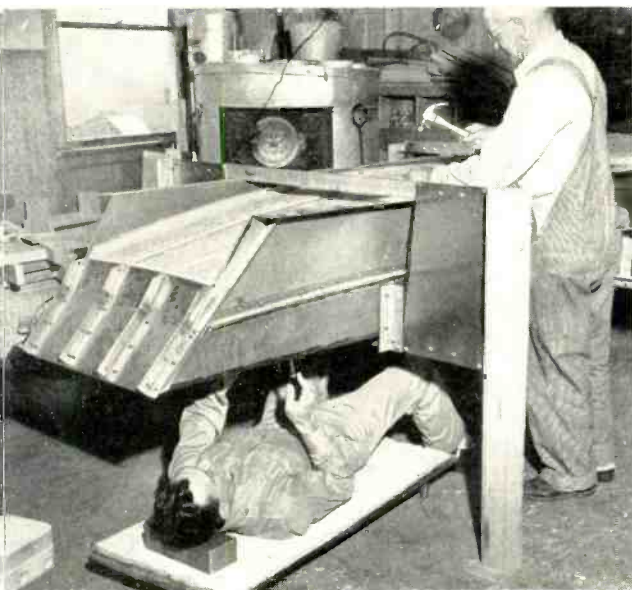
J. Morrell, left, and W. E. Thomsen, right, assemble a section of the reflector for an experimental plywood horn-reflector microwave antenna. The section is removed from the jig after glueing and the reflector lower surface is coated with copper foil.
