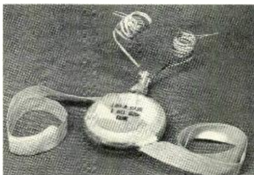
Fig. 2—Program-circuit loading coil.
