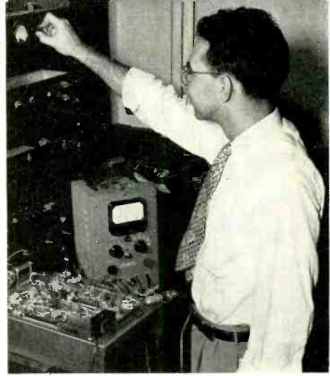
Charlie is measuring voltages on the breadboard model of a pulse forming device that he built.
