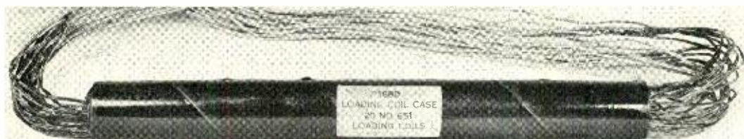
Fig. 5—A twenty-coil assembly employing a new coil for loading long subscriber lines.
