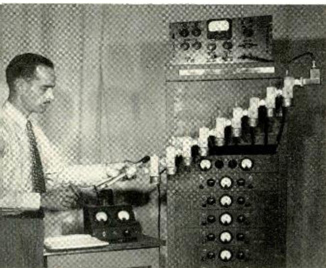
E. L. Chinnock holds a fluorescent lamp noise generator in his left hand preparatory to a measurement of noise figure of an experimental amplifier.
