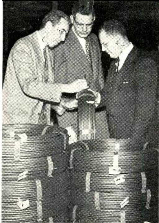
“...Neoprene makes an entirely satisfactory tough and long life jacket for drop wire...” C. C. Lawson (left) examines a roll of Neoprene drop wire with C. B. Clotworthy (W. E.) and G. N. Vacca.
