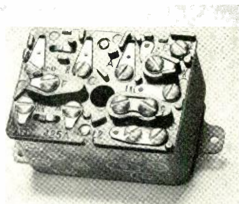
Fig. 5—Cover of 425A network was designed to make connections simple and accurate.
