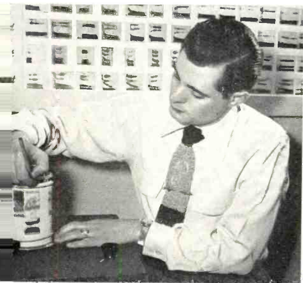
Left—By means of filters, the sound spectrograph breaks a sound up into its dominant frequency groups. Then by means of an electric spark, it plots (burns) each group as a shaded bar on a rotating paper cylinder with low frequencies at bottom, higher ones above. Here, an interval of special interest in a subject's spectrogram is being marked for further study. For ready reference, spectrograms of typical speech sounds are mounted on the wall.
