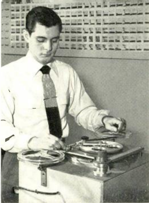
A. J. Prestigiaco adjusts the magnetic tape record of the model sounds transmitted to a loudspeaker in the free space room. Each sound is repeated at 2.5 second intervals.
