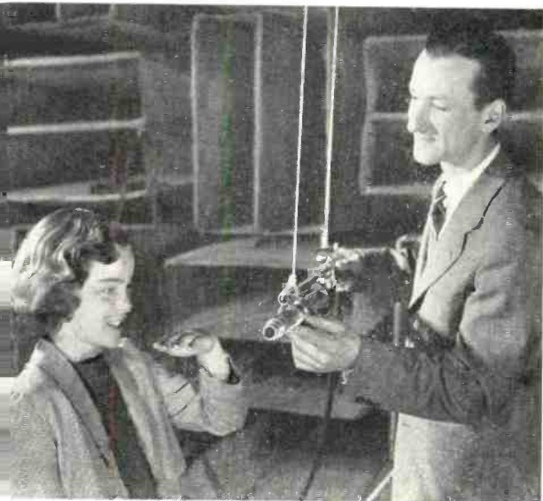
Below—To isolate clues to recognition of word-sounds, data must be plotted in three dimensions, which is difficult to do on paper. Knitting needles stuck through graph paper mounted on cork provide a quick, flexible plotting method. Two of the dimensions are supplied by the paper, the third by the height of the needle. Each group of needles applies to a distinctive vowel sound.
