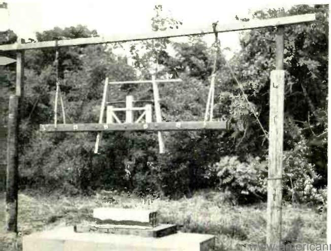
Vitrified clay conduit, used to house underground cables, is often subjected to shocks in shipping, handling, and installation, which may result in breakage if the conduit is not strong enough to withstand them. Consequently, resistance to shock is an important consideration in evaluating changes in design, materials, or manufacturing processes.
