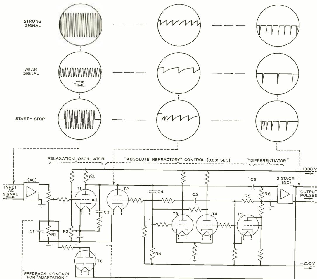
Fig. 2—Schematic of the analog "hair cell" pulsing circuit, with illustrations of several sample wave forms of the operating voltages.
