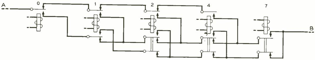
Fig. 1—One form of checking circuit used with the new five-element code.
