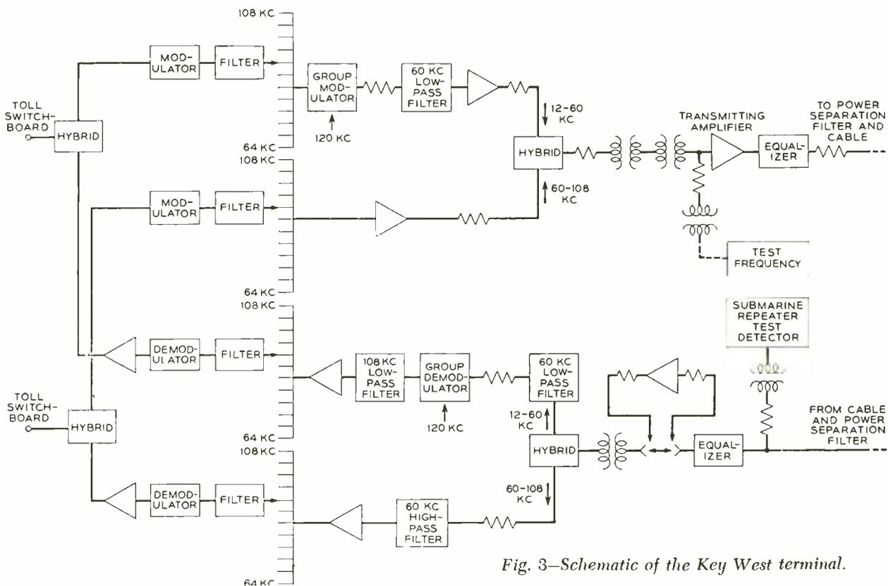
Fig. 3—Schematic of the Key West terminal.
