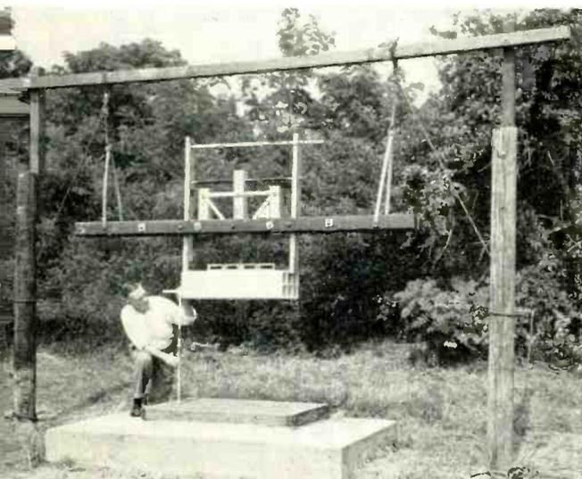
Fig. 1—J. H. Gray checks the height of fall of a six-duct conduit after it has been carefully leveled.
