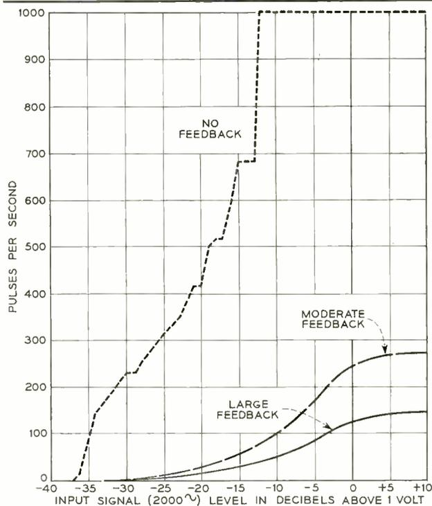
Fig. 3—Response characteristics of the analog “hair-cell” pulsing circuit.
