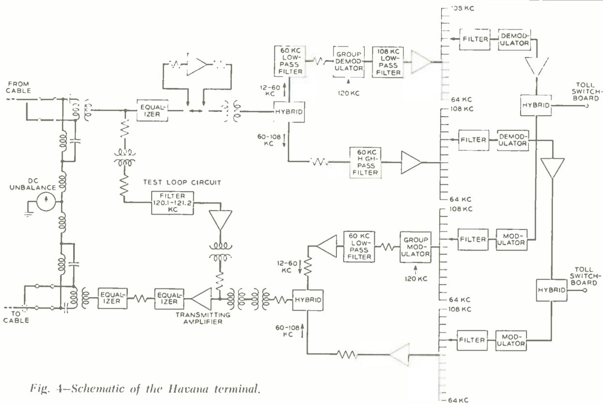
Fig. 4—Schematic of the Havana terminal.
