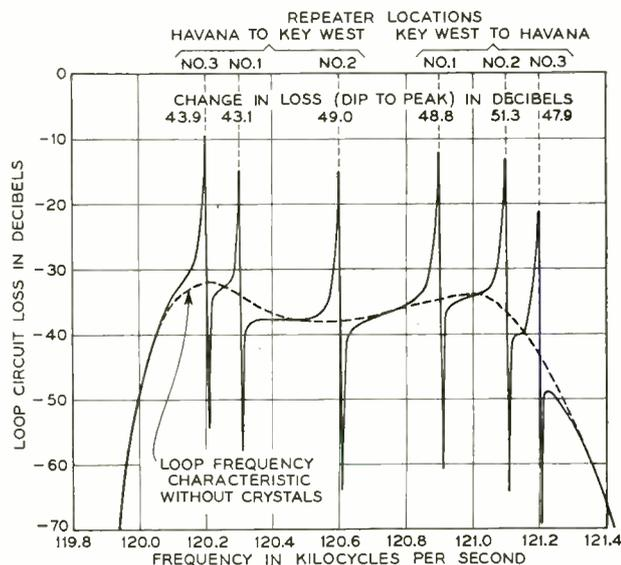
Fig. 2—Measured transmission characteristics of test frequency loop circuit showing the crystal peaks and dips. Tube performance of a particular repeater is indicated by the difference between its peak and closely adjacent dip loss.
