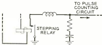
Fig. 4—Contact protection for the 268 relay.
