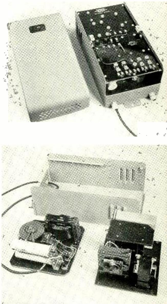
*Fig. 2—The J86731A, List 2, power-supply unit furnishes the same low-voltage dc and ac by the same unit—shown at the left of the lower photograph—as does the List 1. In addition—by means of the unit at the lower right, it supplies 20-cycle signaling current.*
