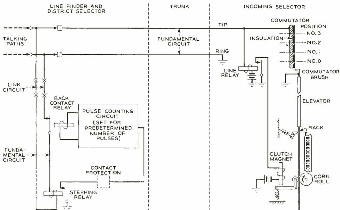
Fig. 2—Schematic of the fundamental circuit of the panel system. The stepping relay is shown at the lower left.
