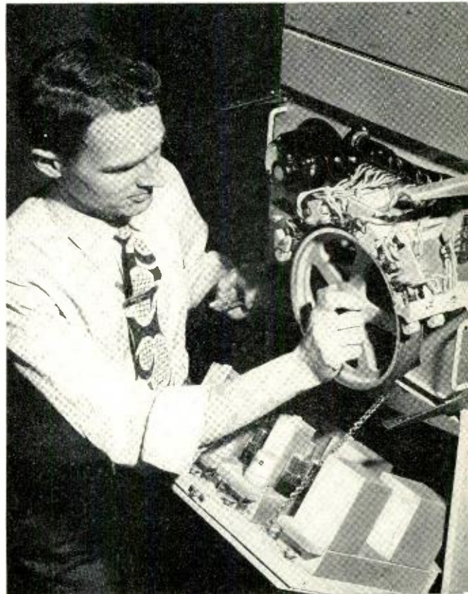
Fig. 1—J. A. Lehans removes wheel of delay quote recorder to inspect magnetic rubber band which accommodates as many as six recordings. Three of the channel amplifiers and associated power supply appear in the tray below.
