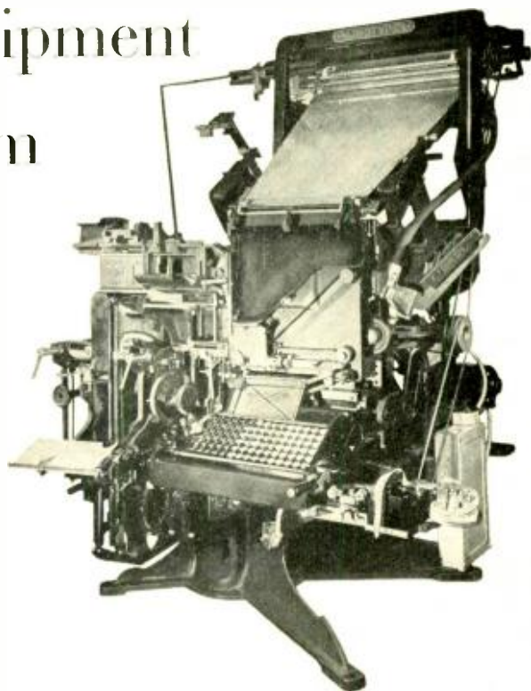
Fig. 1 — A Linotype machine equipped with a Teletypesetter control unit, evident at the right with the keyboard.
