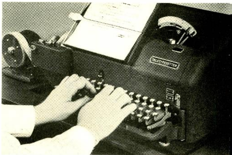
Fig. 2 — The Teletypesetter perforator.
