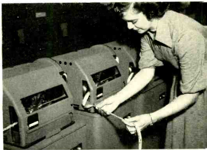
Intercept machines used to hold information not immediately deliverable as a result of maintenance or repairs at the addressed station.
