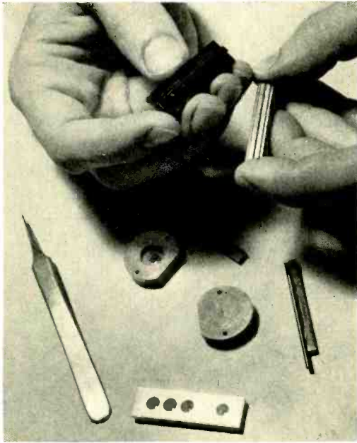
Fig. 2—Parts used to form the interdigital waveguide section showing the relative sizes of the various units.
