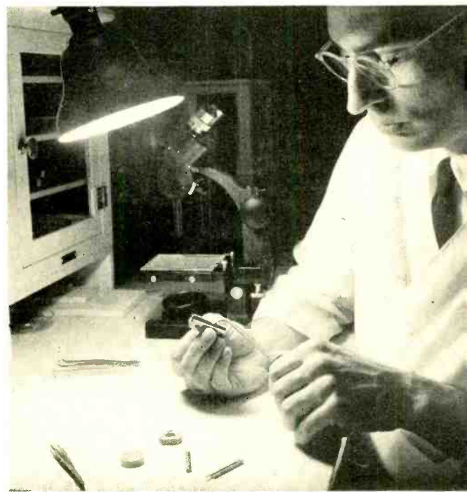
Fig. 6 — The author preparing the surfaces of an interdigital waveguide section.
