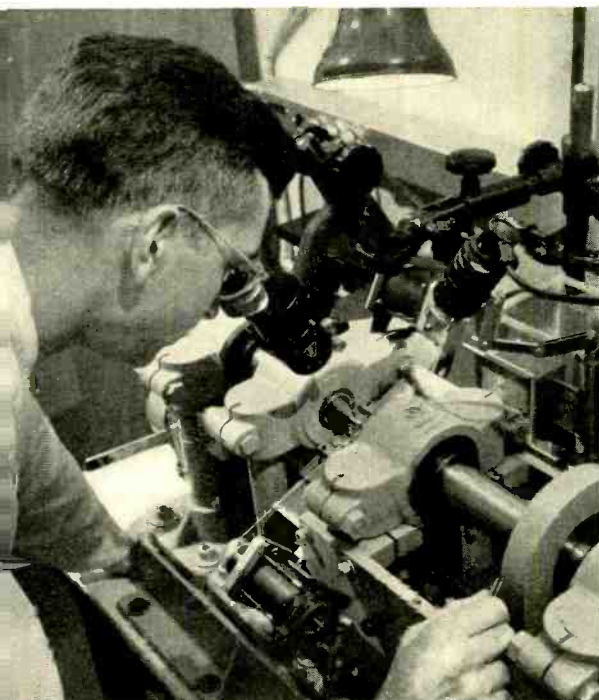
Fig. 5 — The author winding a helix for the hairpin tube.
